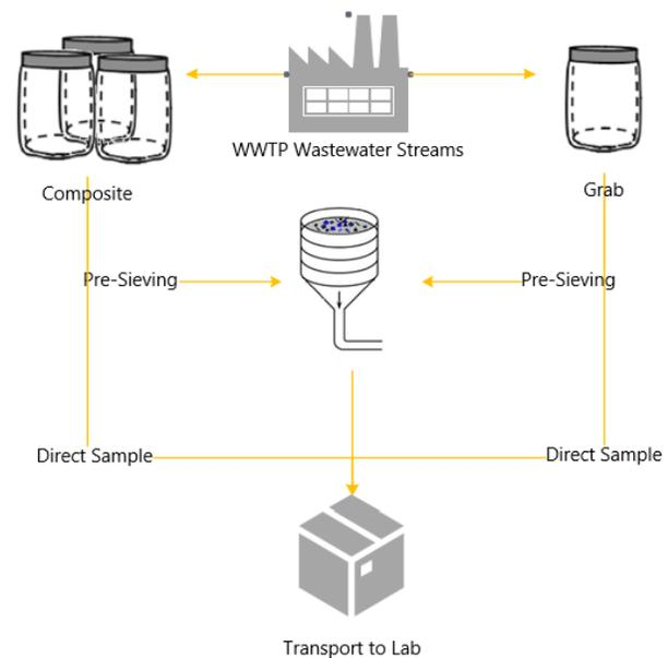
Figure 5. Microplastic in Wastewater Sampling Methods Flowchart (adapted from Bayo et al., 2021, and Long et al., 2019)
