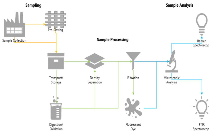
Figure 3. Flow Diagram for Common Microplastic in Wastewater Testing Methods
