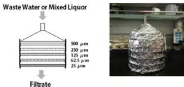
Figure 6. Covered stacked sieve sampling device (reproduced from Lv et al., 2019)
