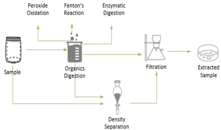
Figure 8. Microplastic in Wastewater Sample Processing Methods Flowchart (adapted from Bayo et al., 2021, and Ben-David et al., 2021)
