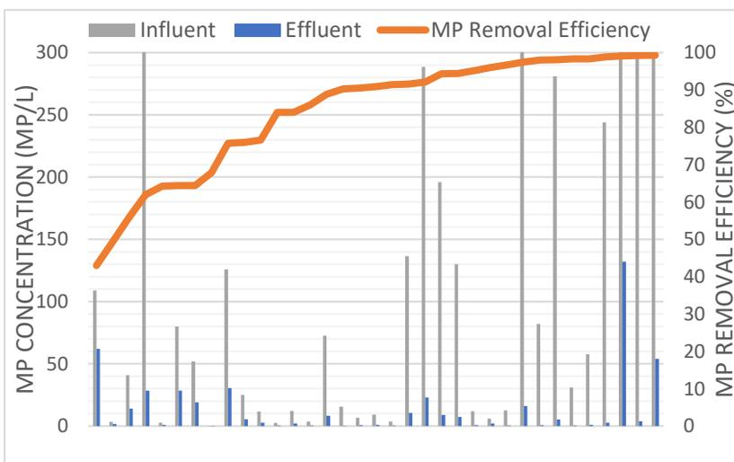
Figure 4. Reported Microplastic in Wastewater Concentrations Less than 300MP/L and Associated WWTP Removal Efficiencies
