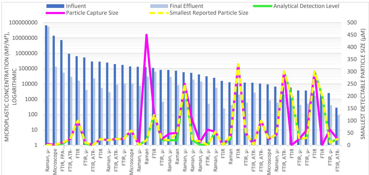
Figure 13. Reported Microplastic in Wastewater Concentrations as Relating to Particle Capture Sizes and Analytical Detection Limits
